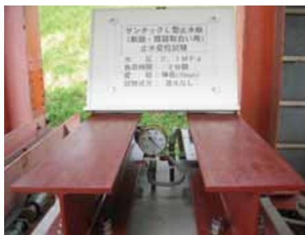
伸び量30mm/耐水圧0.1MPa
