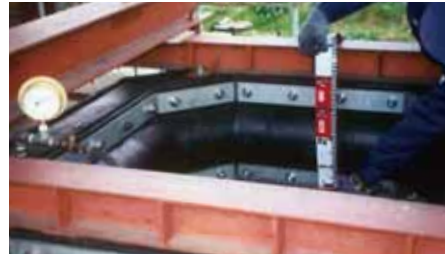
伸び量100mm/耐水圧0.15MPa
