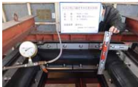
伸び量100mm/耐水圧0.15MPa
